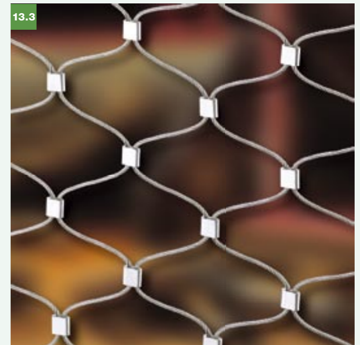
13.3 Webnet with extended mesh angle: when stretched, the wire ropes load the sleeve (breaking limit).
