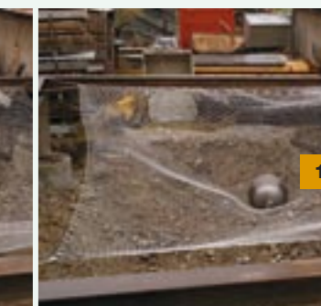
13.3 Webnet with extended mesh angle: when stretched, the wire ropes load the sleeve (breaking limit).
