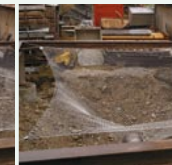
13.3 Webnet with extended mesh angle: when stretched, the wire ropes load the sleeve (breaking limit).
