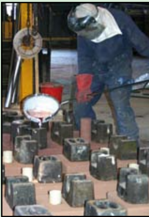
Poring molten aluminium into the mould in the foundry.
