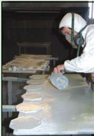
Spraying the basecoat onto plaques.
