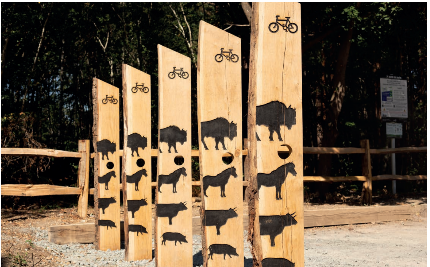
TIMBER THAT INCLUDES WANE, KNOTS, CRACKS AND SPLITS
