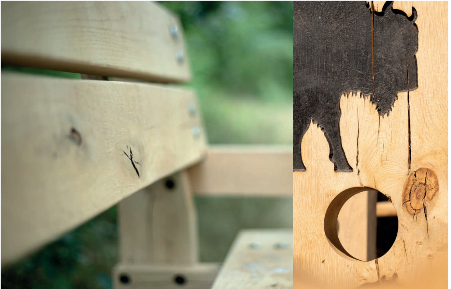
LIVE KNOTS ARE INTEGRAL PARTS OF THE TIMBER WHERE BRANCHES USED TO BE
