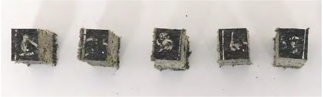
Figure 12 Photograph of compressive strength samples after testing
