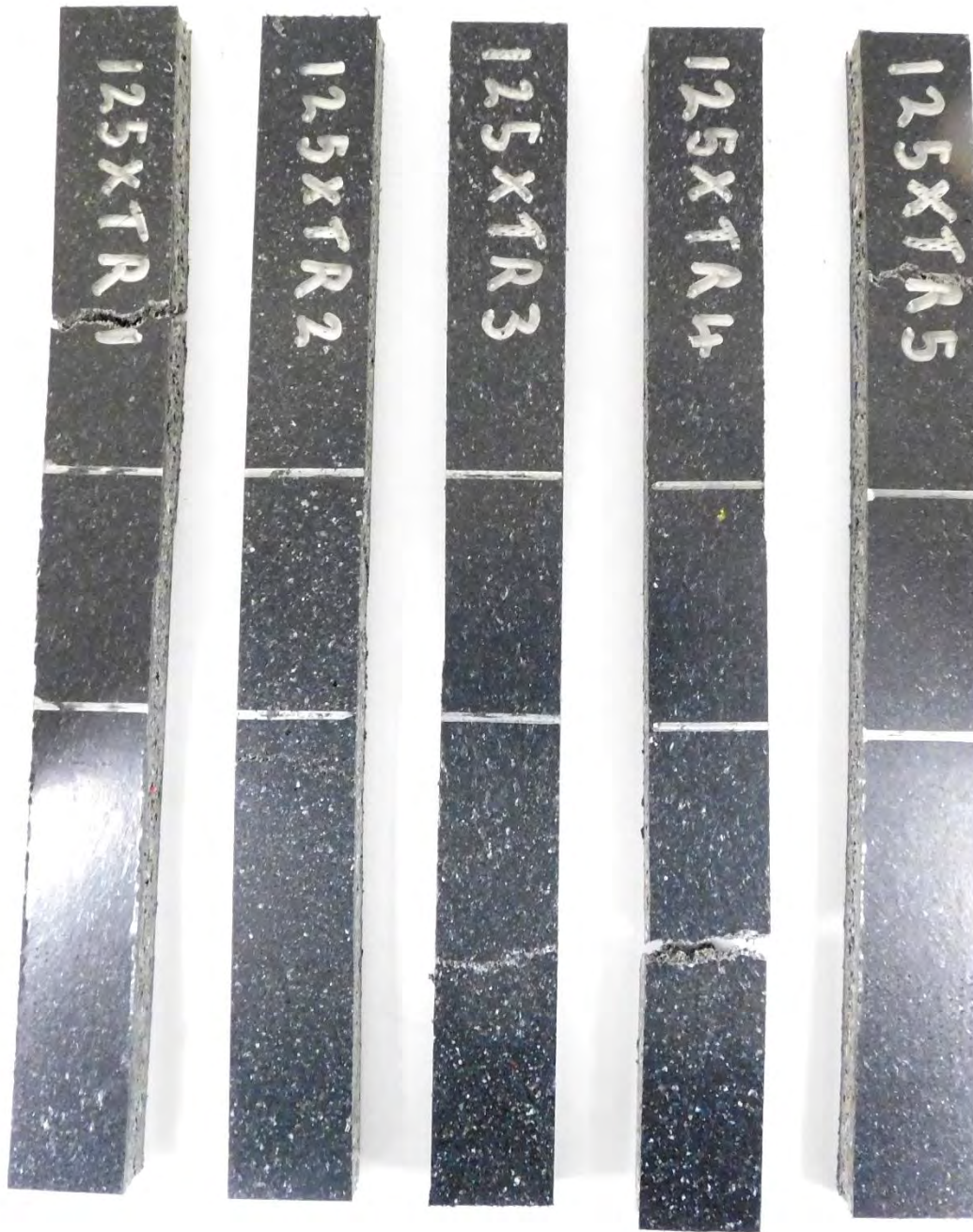
Figure 2 Photograph of tensile samples after testing
