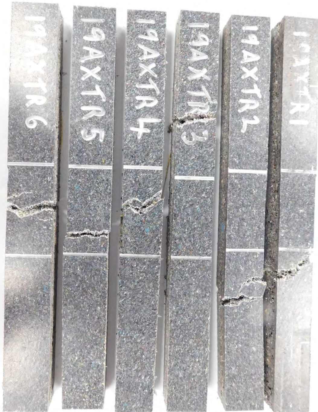
Figure 8 Photograph of tensile samples after testing
