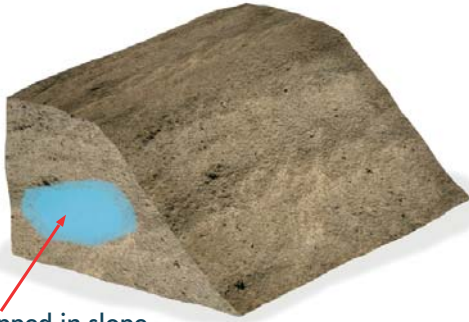
Water trapped in slope
