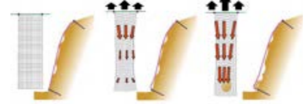
1. Basic case Steelgrid® 2. Mesh weight 3. Weight of the debris
