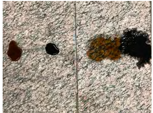
After an hour and a half: Greatly reduced the speed of absorption of the stain into the stone so you have enough time to clean it away.
