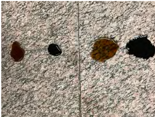
Immediately spilt: Oil and coffee has just been spilt, left side has been protected and the right side is untreated.
