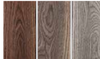
At Installation 6 months + 1 Year +
