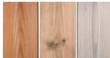
At Installation 6 months + 1 Year +
