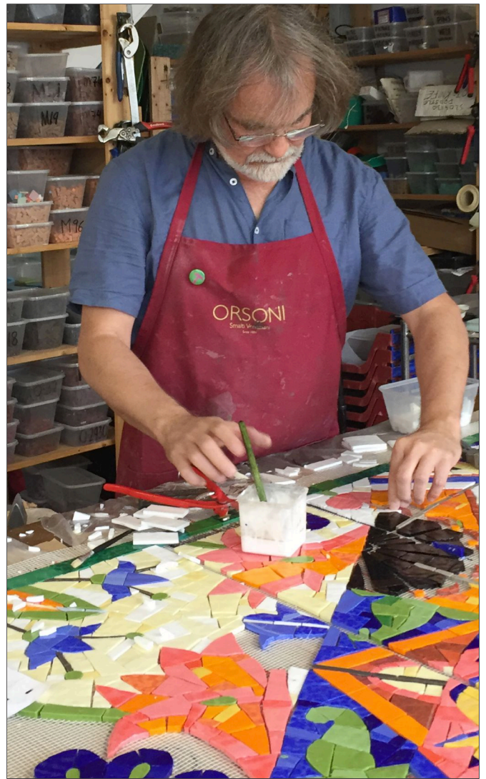
■ Working indirect onto glass fibre net with Smalti Piastrina
