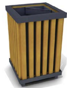
92003 50 litres Outer: 370 x 370 x 670mm (w x d x h) Inner: 300 x 300 x 590mm (w x d x h) Pressure treated softwood / Powder coated aluminium frame / mild steel bin
